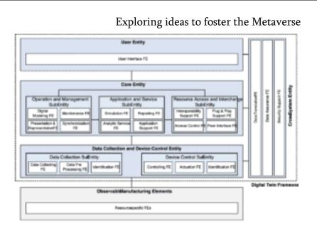
The four layers defined by ISO for the creation and operation of Digital Twin in manufacturing, Image credit: ISO[/caption]
