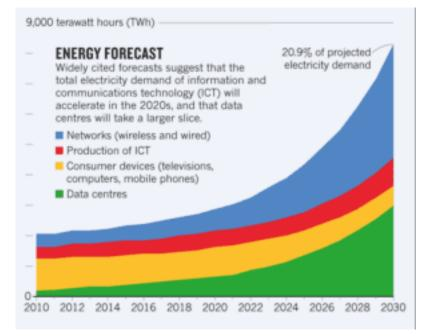
Bits are so "tiny" and weightless we often disregard their impact on energy. The he problem is that the amount of bits is staggering and the equipment needed to manage them is very power intensive. The graphic shows the expected increase in power usage in this decade to manage "bits". As you can see the lion share is taken by networks and by data centres. Image credit: <u>Clarissa Garcia, AKCP</u>
